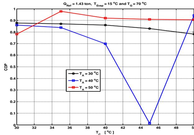
Figure 11: The Relationship between the Coefficient of Performance and the Condenser Temperature
