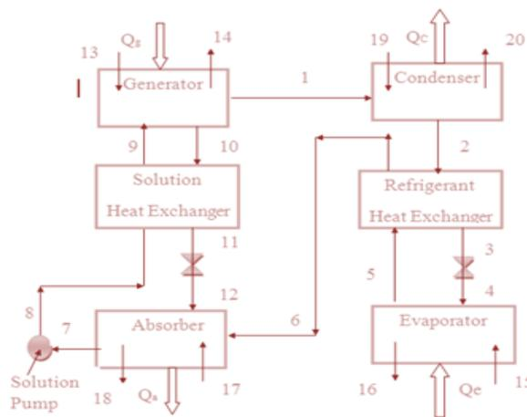
**Figure 6: Schematic Diagram of the Water–Lithium Bromide Absorption Refrigeration System (ARS)**
