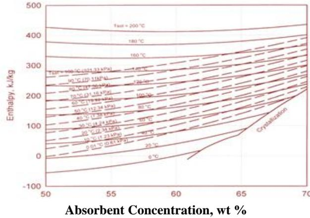
Figure 8: Enthalpy-Concentration Diagram of the H<sub>2</sub>O + LiBr
