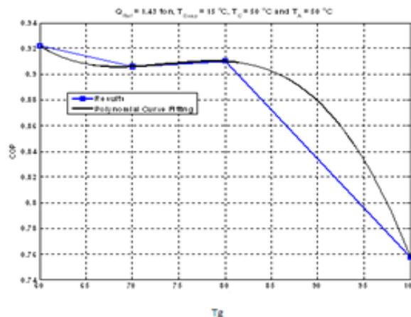
**Figure 10: The Relationship between the Coefficient of Performance and Heat Generator, at  $T_c=T_a=50^\circ\text{C}$**
